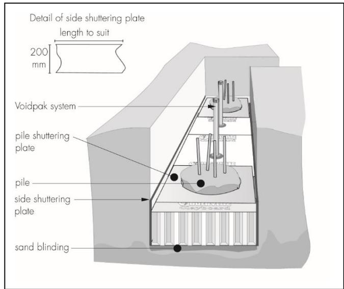
Figure 4 Pile shuttering plate
