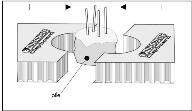
Figure 3 Side shuttering plate
