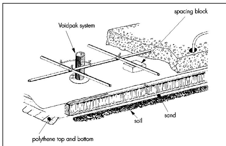
Figure 2 Floor and ground beam details
